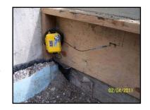
By recording in-situ concrete temperatures, users are able to accurately estimate the in-place strength of the concrete at any point in time. The system is calibrated using strength test samples of the actual mix design in use. In fact, the maturity method has been shown to be SUPERIOR to test samples for in-place strength determination.
